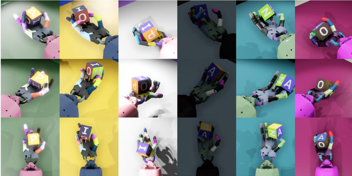
**Fig. 6.** Simulations with different randomized visual appearances. Rows correspond to the renderings from the same camera, and columns correspond to renderings from three separate cameras that are simultaneously fed into the neural network.
